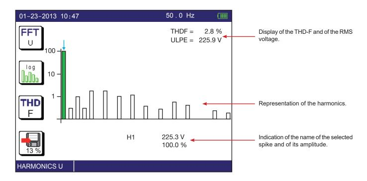
The frequency and amplitude of the selected harmonic (in green) are indicated at the bottom of the graph. To select another harmonic, use the ◀ ▶ keys. The device then shifts from the fundamental (H1) to harmonic H2, then to harmonics (H3, H4, ..., H25). And on the next page it sweeps the harmonics from H26 to H50.
