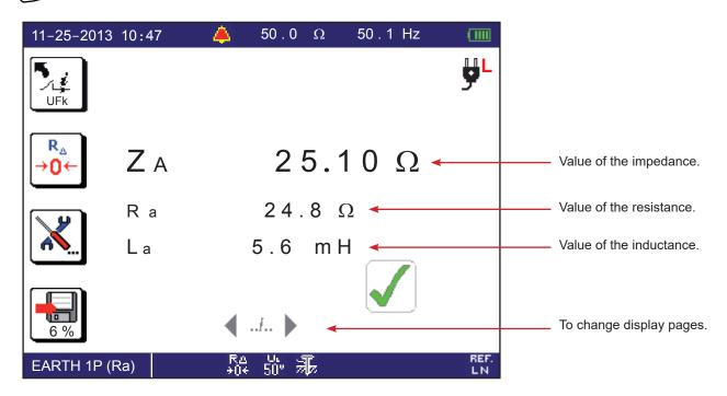
The third page displays the values of  $Z_s$ ,  $R_s$ ,  $L_s$ . The fourth page displays the voltages  $U_{LN}$ ,  $U_{LPE}$ ,  $U_{NPE}$  and on the rod ( $\nearrow$ ) before the measurement.
