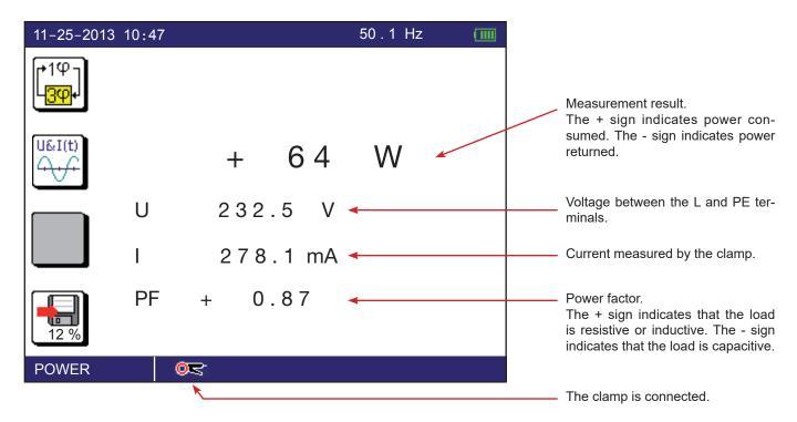
If the phase of the current with respect to the voltage is not correct, turn the clamp around, with the help of the arrow marked on the jaws, in order to reverse the phase by 180°.
