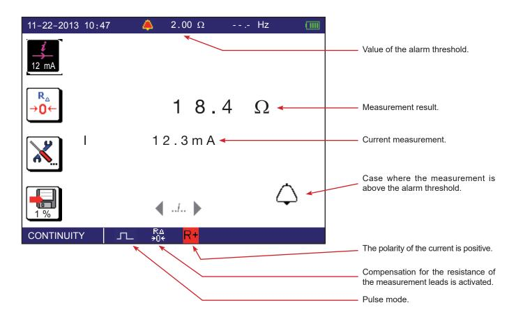
In the case of a resistance measurement (kΩ), there is no current reversal and no compensation for the measurement leads.
