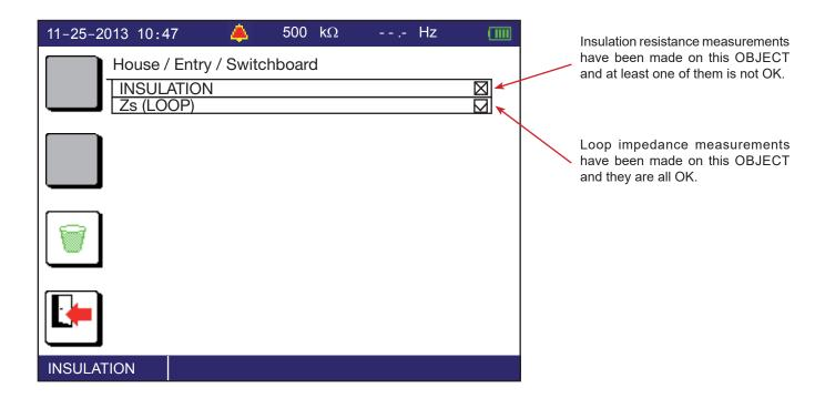
Press the **OK** key to expand a TYPE OF **TEST**.
