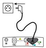
In the Zs (R<sub>A</sub>/S<sub>EL</sub>.) and RCD, settings, the device also indicates the position of the phase on the display unit using the symbol. The mains socket outlet of the measuring cable is marked with a white reference spot.
