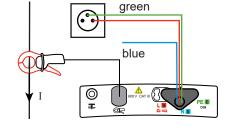
■ The current measured by the clamp is too high. Use a clamp having a higher ratio.
