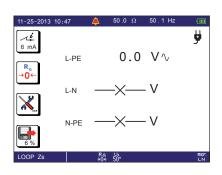
If  $U_{N-PE}$  does not display -x --, the protection in the N terminal has been activated.
