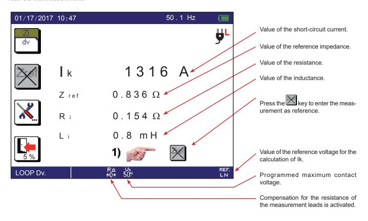
Change the connection as explained above and press the **TEST** button again to make the second measurement. After the second measurement:
