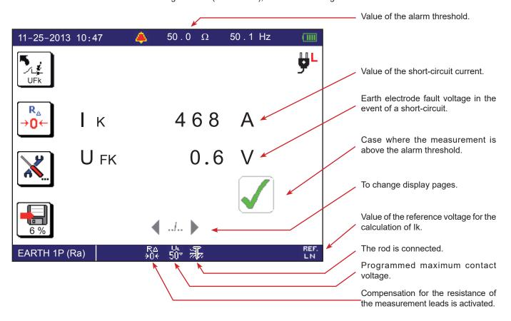
$U_{Fk}$  is calculated only in earth measurement on live circuit with a high current (TRIP mode).  $U_{Fk} = Ik \times Z_A$ .
