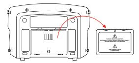
3. Then push the screwdriver towards the rear and the battery slides out of its compartment.
