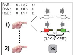
Connect the three leads that you are going to use for the measurement to the L, N, and PE terminals, short-circuit them, then press the **TEST** button.
