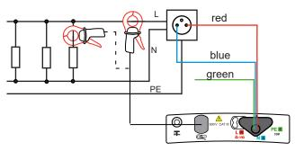
In the case of a three-phase network balanced in voltage and in current, connect the measuring cable terminated by 3 leads to the device and to two of the three voltages  $U_{12}$ ,  $U_{23}$  or  $U_{31}$  using the red and blue leads. Then, with the clamp, surround the conductor of the third phase  $I_3$  (for  $U_{12}$ ),  $I_1$  (for  $U_{23}$ ) or  $I_2$  (for  $U_{31}$ ).
