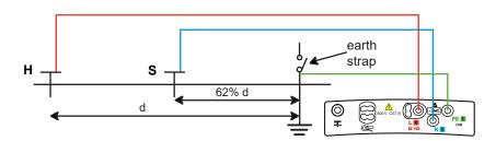
Connect the cables to the H and S terminals. Power down the installation and disconnect the earth strap. Then connect the E terminal to the earth electrode to be checked.
