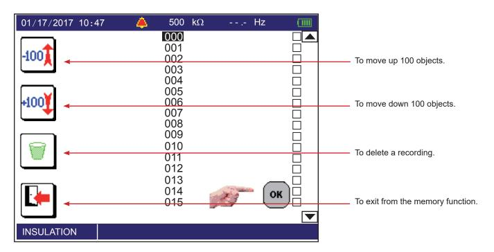
Use the ▲ ▼ arrows to select the object in which you want to record your measurement and validate by pressing the OK key.
