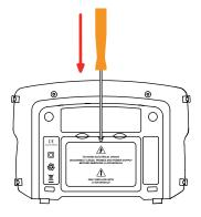
2. Turn the device over and insert a screwdriver into the hole in the battery pack.
