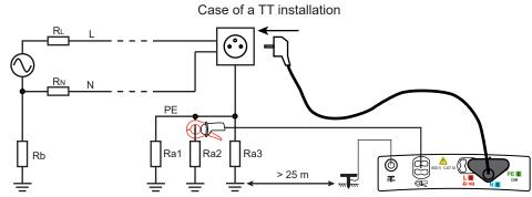
For a more accurate measurement, you can choose a high current (TRIP mode), but the RCD that protects the installation may trip.
