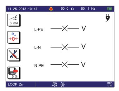
If  $U_{L\text{-PE}}$  does not display -x --, the protection in the L terminal has been activated.
