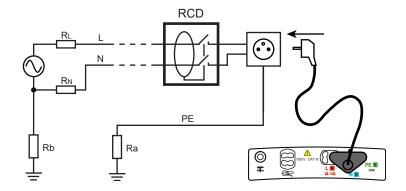
If possible, first disconnect all loads from the network on which you test the RCD. This prevents interference with the test by any leakage currents due to these loads.
