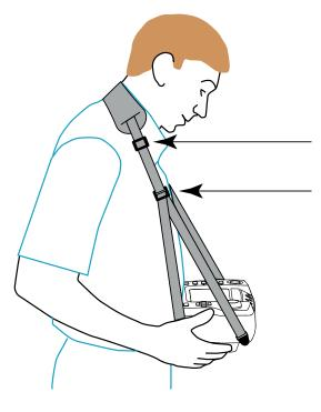
The 4-point hands-free strap will let you use the device while leaving your hands free. Snap the four fasteners of the strap onto the four lugs on the device
