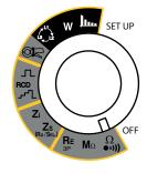
Use the leads to connect the device to be tested between the  $\Omega$  and COM terminals of the device. The object to be tested must not be live.
