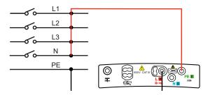
If the insulation is not sufficient, you must then make the measurement between each of the pairs to locate the fault. It is for this reason possible to index the recorded value with one of the following values: L-N, L-PE, N-PE, L1-PE, L2-PE, L3-PE, L1-N, L2-N, L3-N, L1-L2, L2-L3 or L1-L3
