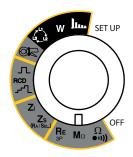
Use the leads to connect the device to be tested between the COM and  $M\Omega$  terminals of the device. The object to be tested must not be live.
