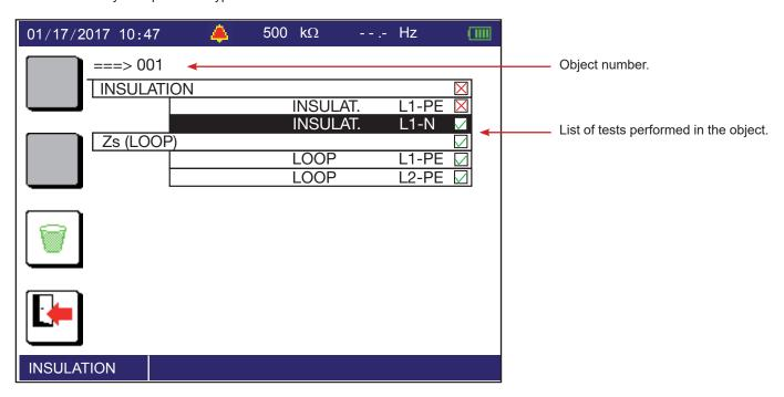
Use the ( ▲ ▼ ◀ ▶ ) keys to select a measurement. Press the **OK** key again to see the recorded measurement.
