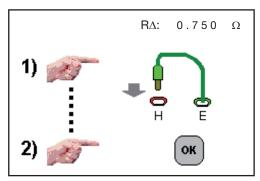
Connect the lead that you are going to use to connect the E terminal to the earth between the H and E terminals, then press the **TEST** button.
