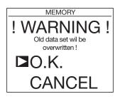
Pressing the MEM key again stores the current measurement results at the selected address. All information about a measurement will be stored at a single location in memory: date, time, test mode and voltage, insulation resistance, capacitance, residual current, and, possibly, DAR, PI, DD, resistance referred to the reference temperature, etc.
